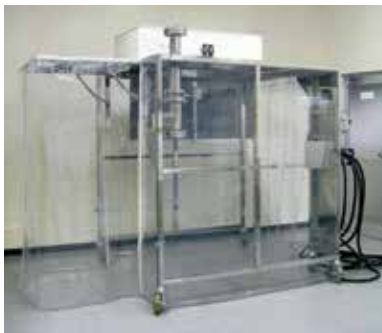
Explosion-proof clean booth
